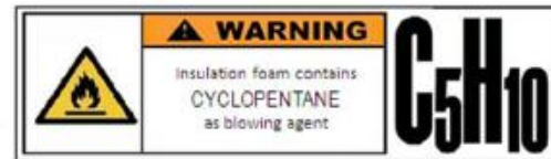
Figure 7-3 Example of marking of the flammable insulation blowing agent
